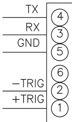
**FIGURE 3.5 - TRIGGER WIRING**
