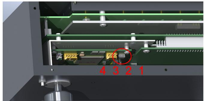
**FIGURE 3.6 - DIP SWITCHES**
