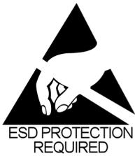
**CAUTION! ESD PROTECTION REQUIRED.** The proper use of grounded work surfaces and personal wrist straps are required when coming into contact with exposed circuits to prevent static discharge from damaging sensitive electronic components.
