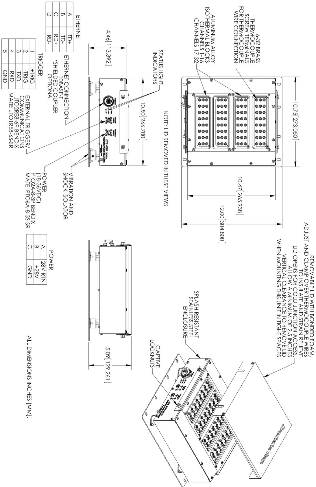
FIGURE 1.1 - PHYSICAL SPECIFICATION, DTS4050/32TX, SCREW TERMINAL INPUTS
