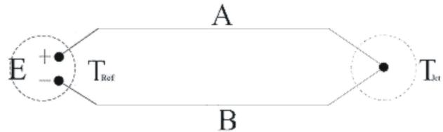
When more than one thermocouple is to be measured, each thermocouple should be two continuous wires between the measuring and reference junctions. This is the most common circuit for thermoelectric testing.
